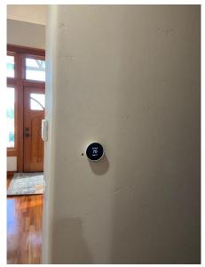
Nest Thermostats don't have a touch screen. Use the touch bar on the right side to control your thermostat. Swipe up to raise the temperature, swipe down to lower it, and tap to confirm. The display will show you how many minutes until your desired temperature is reached.
